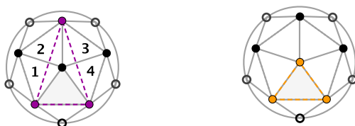
Figure 20. Left the schematic representation of an obtuse vertex of the long tile, right an acute vertex of the long tile always together with 15 of the 20 possibilities to build a long tile seen from its acute vertex
